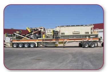
Portable Closed Circuit Crushing Plant with Metso HP300 cone and Metso 6x20TD Screen, (1) 60" under screen conveyor, (1) 18" top cross conveyor, (1) 24" bottom cross conveyor, (1) 42" feed conveyor with hydraulic fold, (1) 42" under crusher conveyor, (1) 36" cross conveyor and (6) leveling jacks
