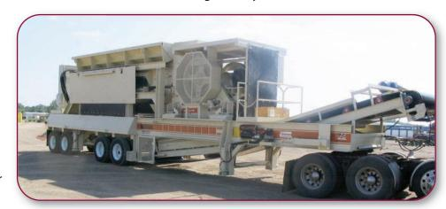
Portable Crushing Plant with Metso C106 Jaw, 58"x20' vibrating grizzly feeder and 48" front discharge conveyor
