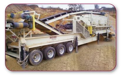
Portable Cone Plant with Cedarapids MVP 380 cone, Cedarapids 6x20TD screen, (1) 60" under screen conveyor, (1) 18" top cross conveyor, (1) 24" bottom cross conveyor, (1) 42" feed conveyor, (1) 36" under crusher conveyor, and (1) 36" rear cross conveyor, and **MASABA** "Brute" run-on jacks
