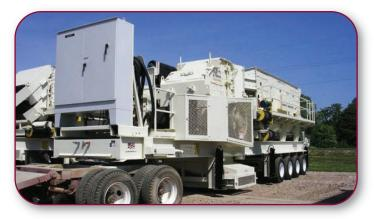
Portable Crushing Plant with Cedarapids 5048 secondary impactor, Cedarapids 6x20TD screen, 48" fold-up side discharge conveyor, (2) 24" side discharge conveyors, and **MASABA**. "Brute" run-on jacks
