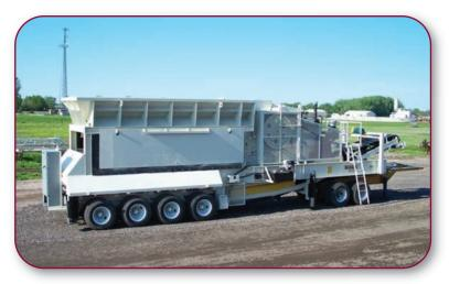
Portable Crushing Plant with Cedarapids 3042, 58"x20' vibrating grizzly feeder and 48" front discharge conveyor
