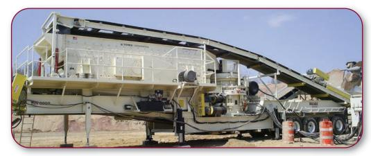
Portable Closed Circuit Crushing Plant with Cedarapids MVP 280 cone, Cedarapids 6x20TD Screen, (1) 60" under screen conveyor, (1) 18" top cross conveyor, (1) 24" bottom cross conveyor, (1) 42" feed conveyor, (1) 36" under crusher conveyor, (1) 36" rear cross conveyor, and **MASABA** "Brute" run-on jacks
