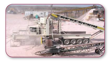
Portable Open Circuit Cone Plant with Cedarapids MVP550 cone, dual 250HP drive, 48" hydraulically folding side discharge conveyor and hydraulically adjustable 42" feed conveyor, and **MASABA** "Brute" run-on jacks
