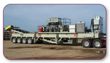
Portable Crushing Plant with Raptor Excel 400 cone, (1) 42" discharge conveyor
