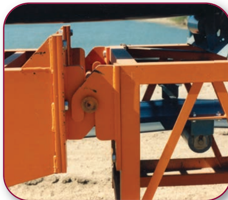
Overland Conveyors in 100' sections with easy joint attachment for quick assembly
