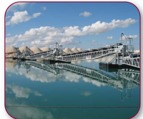
Qty (6) 36" x 100' Floating Pontoon Conveyor System
