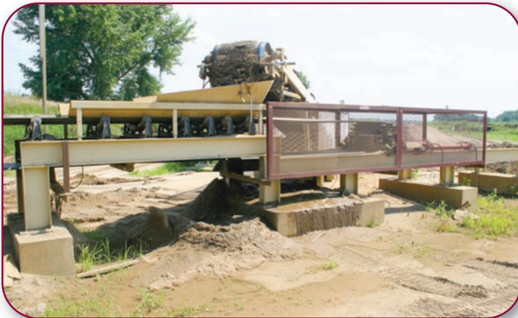
36" x 1900' Overland Conveyor feeding a 36" x 400' Overland Conveyor
