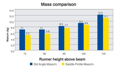
Using Saddle Top frames, the mass of the screen frame reduces, improving the G-Force produced by the screen drive.
