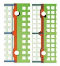
This illustration shows how the Saddle supports the internal frame of the modular screen panel, increasing panel life.
