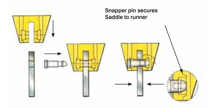
The polyurethane Saddle Top is a replaceable ex-stock item that can be changed in the same time as a modular screen panel.
